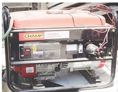
Portable generator set – a 'genset'
