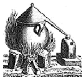
The first type of still was called an Alembic, although this properly referred to the cap with a spout that sat on top of the boiling vessel. It worked well, and with variations to make use of modern materials is just what you need to distil botanicals. The second is reminiscent of the moonshine contraptions still used (and raided) in America, but without the cooling 'worm' so characteristic of them.
