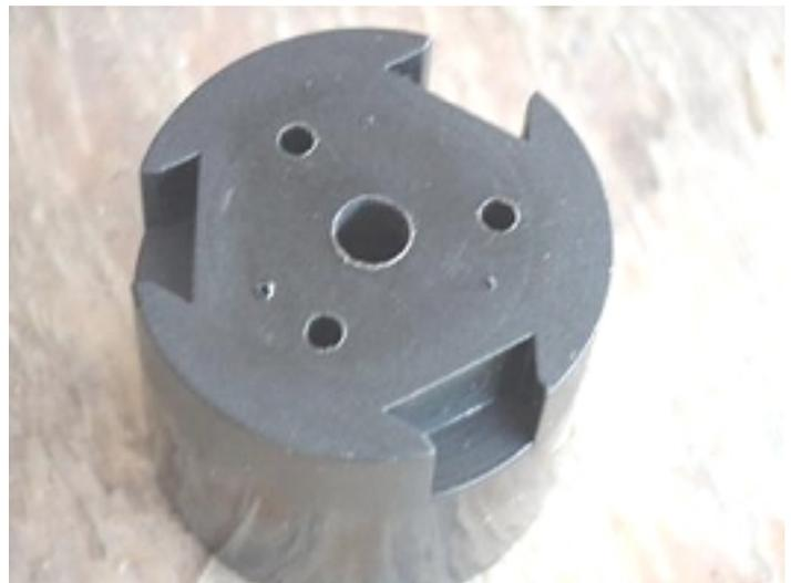
Completed anemometer hub assembly
