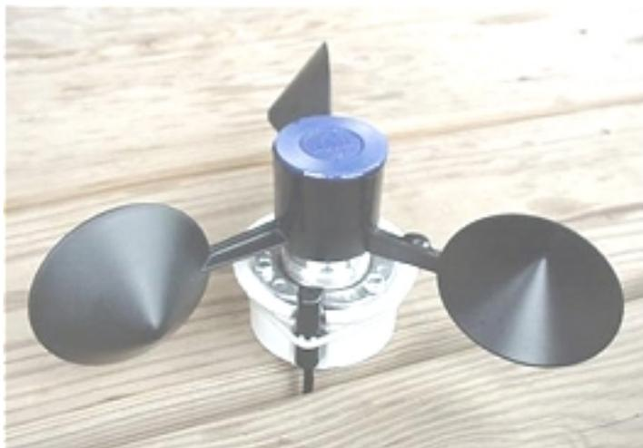
Completed anemometer cup and sensor assembly
