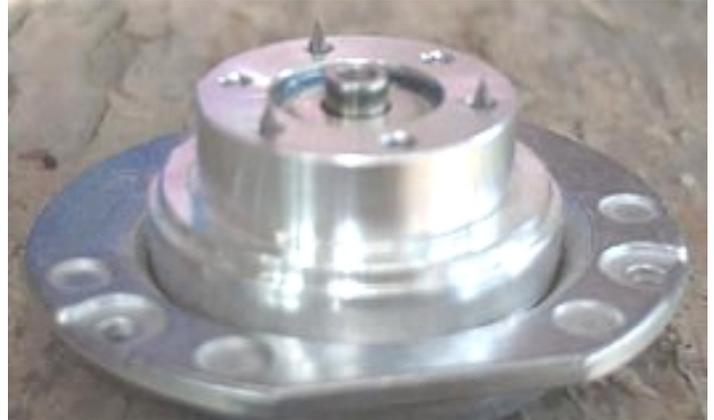
Nails in Motor for marking hub holes
