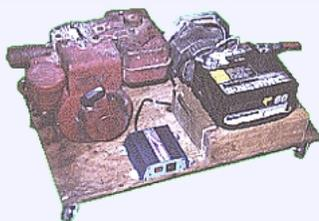
Want your own Emergency Generator? We have put together a kit which includes a 3hp vertical shaft gasoline engine, 94 amp alternator, mounting bracket, 4" pulley, V-belt, battery cables, 115ah deep cycle battery with case, 700 watt inverter, and mounting base with casters. You
